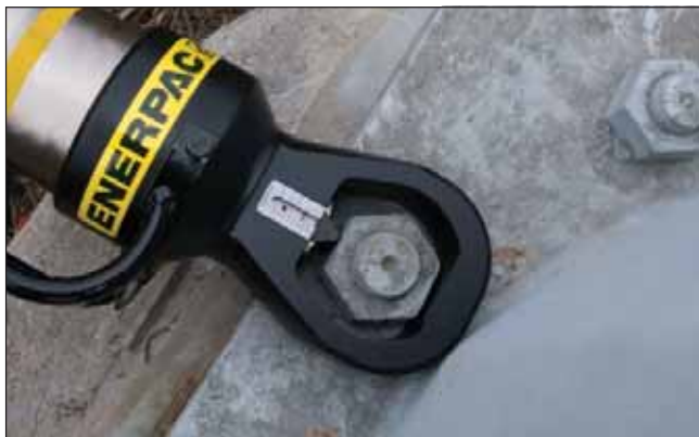
◀ Heavily corroded and weathered nuts are quickly split and removed using an NS-Series Nut Splitter.
